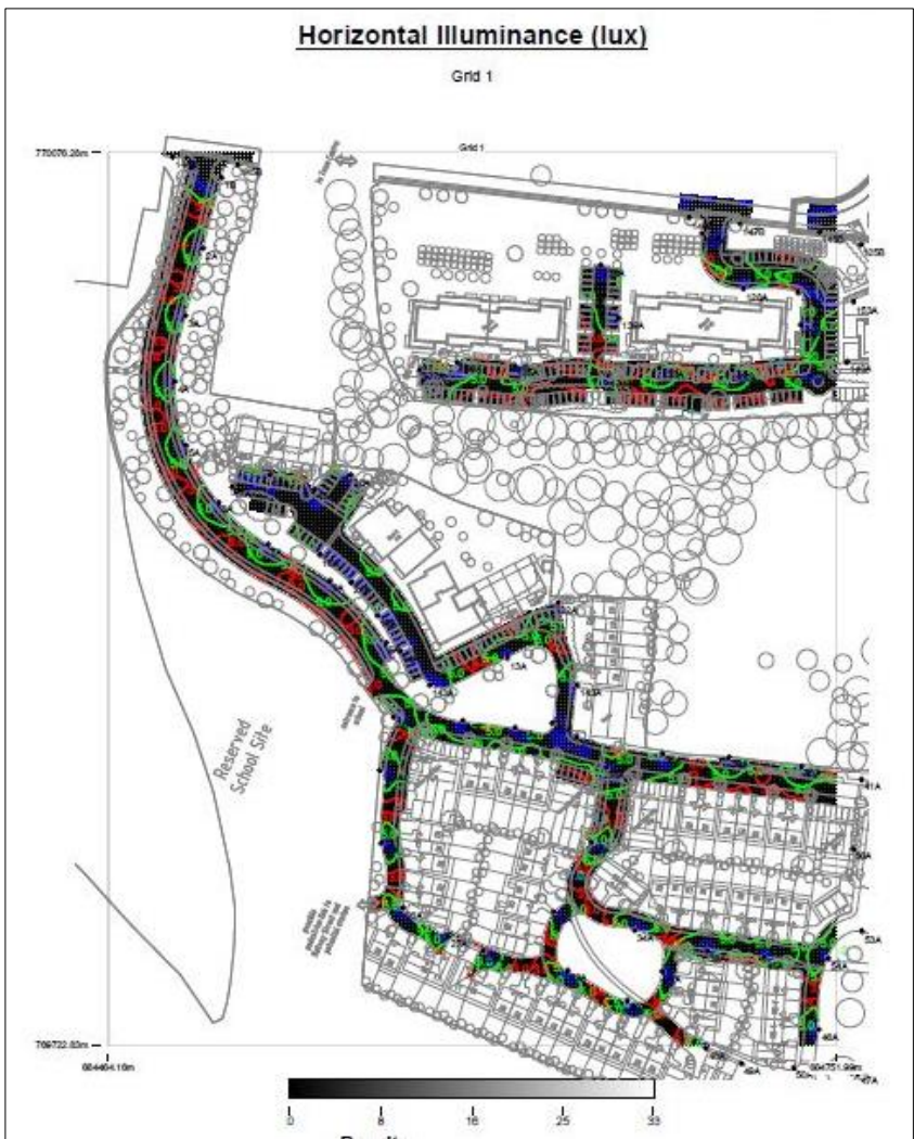
Figure 11a: Horizontal Illuminance levels for Grid 1.
